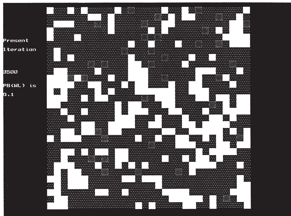
Figure 2. A dynamic simulation of 100 solutes and 2000 water molecules in a 55 \times 55 grid. The figure enlarges a section of the total grid space. The P_B(WL) value is 0.10. The black cells are water, the gray are solute and the white are cavities.
